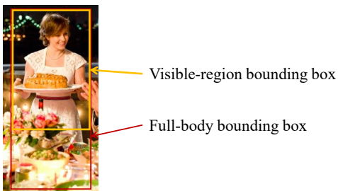
Figure 6: An illustrative example of visible-region bounding box and full-body bounding box annotations.
